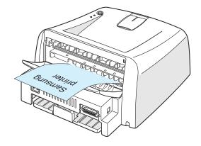
Printing from the Manual Feeder to the rear output tray provides the **straight paper path**. Opening the rear output tray might improve the output quality with the following:
